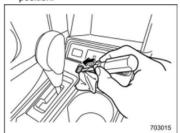
Wrap the tip of a flat-head screwdriver with vinyl tape or a cloth and use it to remove the shift lock cover. The shift lock release button is located under the shift lock cover.
