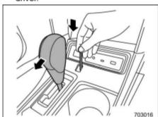
While depressing the brake pedal, insert a screwdriver into the hole, move it right and left while pushing the shift lock release button using a screwdriver, and then move the select lever.
