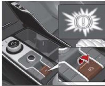
Set the Electronic Parking Brake (EPB)
