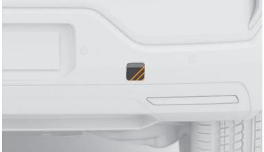
Screw the towing eye all the way into the socket. IMPORTANT It is important that the towing eye is firmly screwed into place. Putting something through the towing eye, such as a wheel wrench, can give extra leverage.
