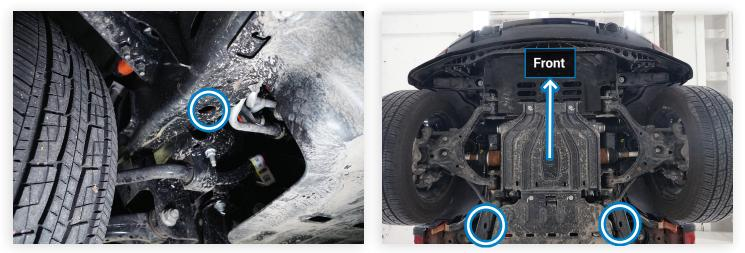
Make connections to the disabled F-150 Lightning at the transport slots in the bottom of the frame behind the sway bar mounts
