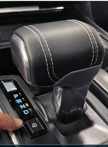
Press brake, shift to Neutral (N), press temporary neutral button twice, turn off vehicle
