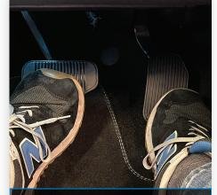
Press brake and accelerator pedals all the way down to unlock shifter
