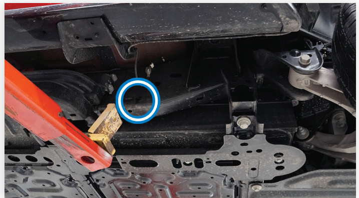
Driver side rear frame rail jacking location
