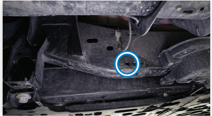
Passenger side rear frame rail jacking location
