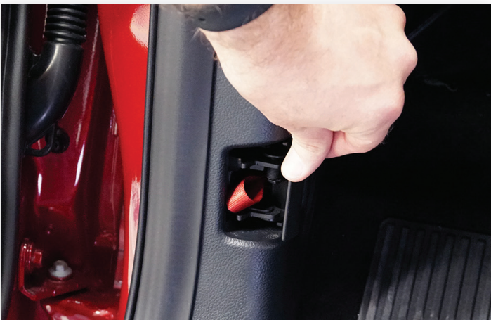
In Driver Side kick panel, pull red tether to open front trunk.
