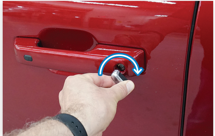
Insert Key Blade in Lock Cylinder. Rotate Clockwise, pull handle to open.
