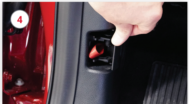
4 Emergency Manual Release - Driver's Kick Panel
