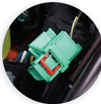
The Low Voltage Service Disconnect should be restored to the ON position and red locking tab pressed down to secure the circuit.
