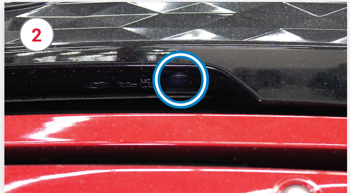
2 Button on Bottom of Grill - Front Trunk
