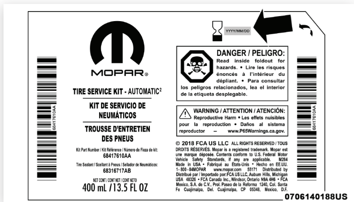
Tire Service Kit Sealant Expiration Date Location
