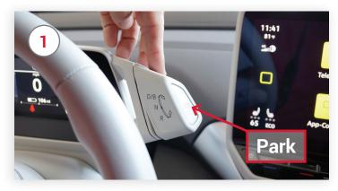
Enter the vehicle with key fob and depress foot brake. Shift vehicle to neutral by pulling the top of the shifter one click towards you.
