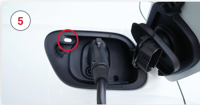
Charge status light will illuminate white, cord can then be unplugged by depressing button on top of the plug.
