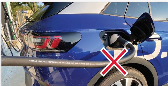
DON'T: The charge cable, especially DC Fast (Level 3), should not be pulled tight or maneuvered in such a way that the connection to the vehicle requires force. This tension the cable is under can potentially make the connector end of the cable wedge inside the charge port requiring additional effort to remove when disconnecting.
