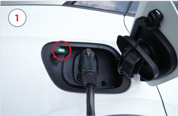
While charging, the charge status light will pulse green and plug cannot be released.
