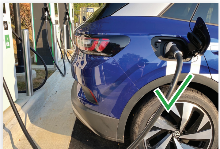
DO: The charge cable should easily reach the charge port. If a connector is not reaching reposition the vehicle.
