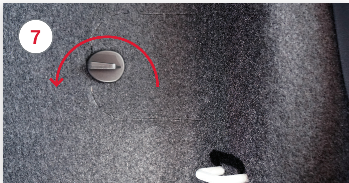
If charge cord cannot be released by either method above, or becomes jammed in charge port, there is a manual release behind an access door in passenger-side inner quarter trim panel in the trunk.
