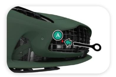
**1.** Insert the tow eye carefully through the grill and install to the exposed female threads (A) until fully engaged against the vehicle body.
