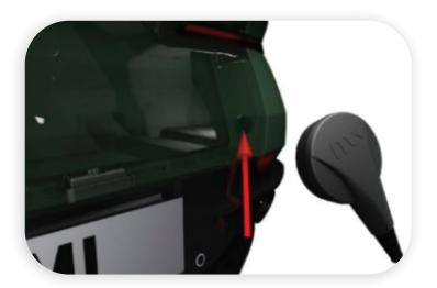
Attach the battery conditioner by guiding it up between the boot and the body (it will attach itself properly with the help from the magnet).
