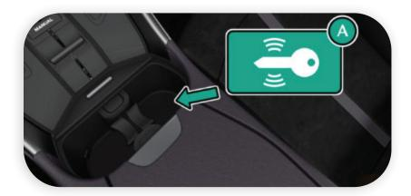
If the vehicle does not start and the message "Place the key in the marked space - See Owner's Manual" is shown in the instrument cluster:
