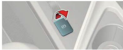
Set the Electronic Parking Brake (EPB)
