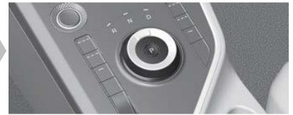
Put the vehicle in P (Park) position by pressing the 'P' button on the rotary shifter
