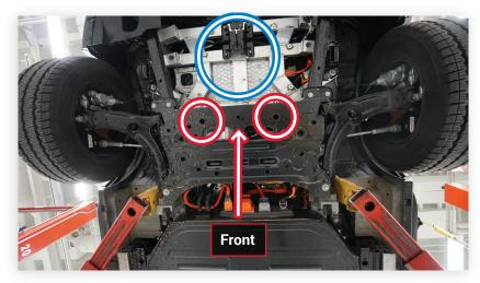
Make connections to the disabled E-Transit at the holes circled in White & Red Short & Long Body variants will have a Spare Tire mounted in place of the White & Blue Circle
