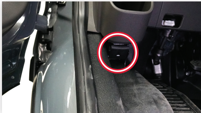
Hood Release is in Driver Side kick panel
