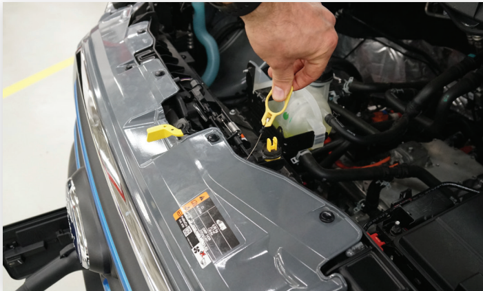
Remove Charge Coupler release ring and gently pull up on cable.
