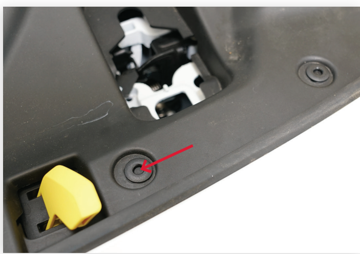
To remove rivets, gently press down on center pin.
