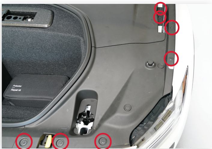
Remove plastic rivets in trim panels, 7 in total.
