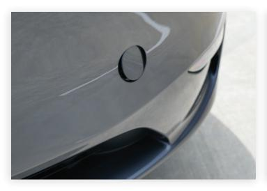
Remove Tow Eyelet Cover to access remote jump leads
