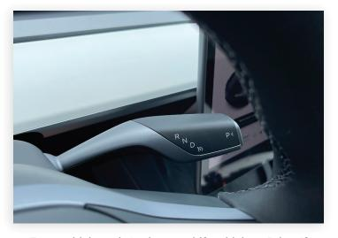
Enter vehicle, wait 2 minutes, shift vehicle to Drive. If vehicle shifts to Drive the Low Voltage battery is being recovered.
