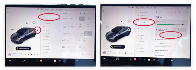
The charge door on the Tesla Model Y can be opened via the touchscreen under the "CONTROLS" menu by tapping the Lightning Bolt or under the "CHARGING" menu by tapping **Open Charge Port**
