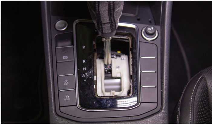
Remove the shifter boot with plastic trim.
