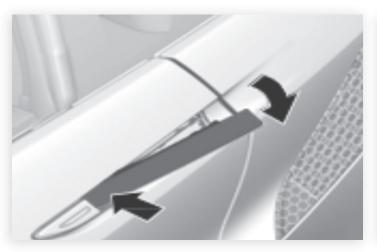
By switching the auto pop-out main switch to OFF, you can disable the auto pop-out function. For the purpose of safety and to prevent damaging the vehicle, disable this function and manually operate the handle, especially when the vehicle is being shipped by train, truck, or boat.
