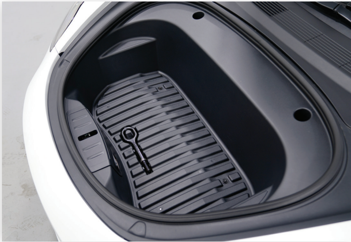
The Tow Eyelet is located in the Front Trunk under the trunk mat.
