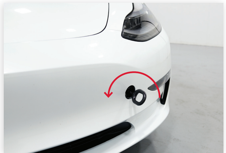
Tow Eyelet is left hand threaded, install counterclockwise until its fully seated in the bumper beam.
