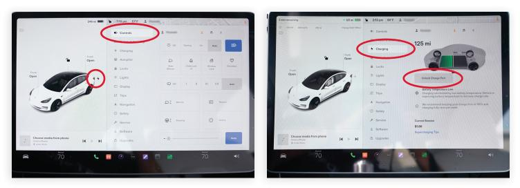
The charge door on the Tesla Model 3 can be opened via the touchscreen under the "CONTROLS" menu by tapping the Lightning Bolt or under the "CHARGING" menu by tapping **Open Charge Port**
