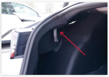
Inside the rear trunk, directly behind the charge port and concealed inside the inner quarter trim panel is a tether to manually release the charge cord.
