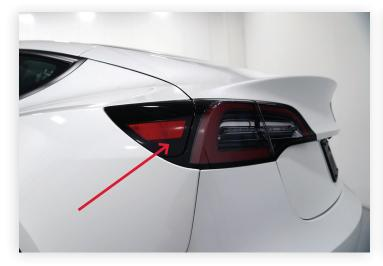
With the vehicle unlocked the charge port door can be opened by pressing it at the bottom
