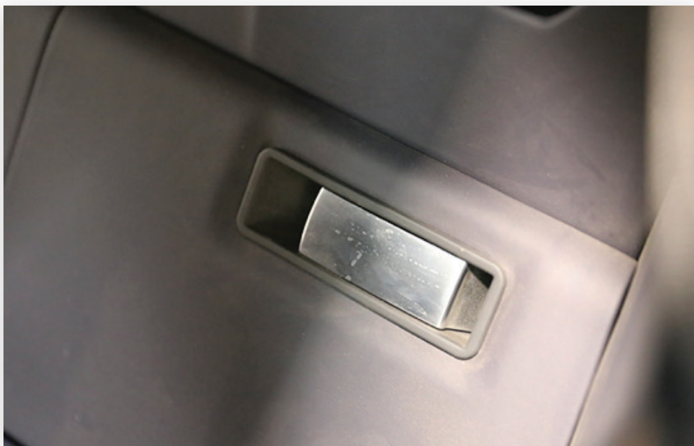
The hood release is located behind the driver's seat on the bulkhead.
