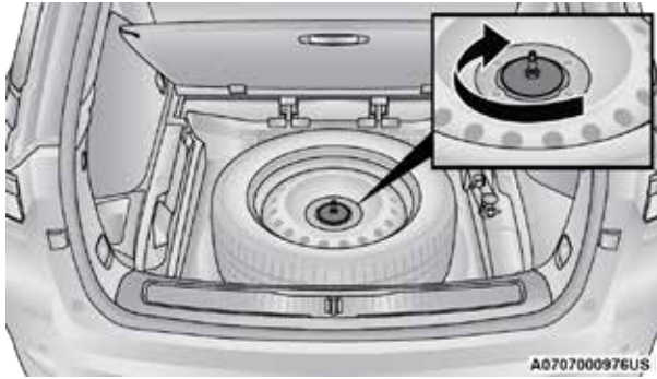
Reinstalling Tire Fastener
